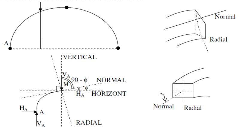
Total force acting along the normal is called normal thrust and total force acting along the radial direction is called radial shear. For the case shown in fig normal thrust
